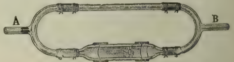
GAULE'S MAXIMUM AND MINIMUM MANOMETER, A, B. (The extremity A is connected with the heart, and B with the mercurial manometer.)
